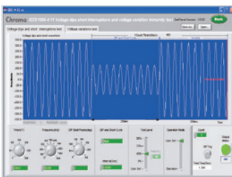
Voltage DIP, Short, Variation Regulation Test
