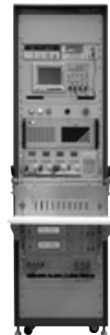
DC to DC Converter ATS
