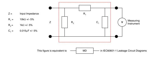
Figure 1.0: Equivalent Circuit - Human Body Impedance
