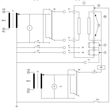
Figure 5.0: Patient Leakage – F-TYPE Applied Part to Ground (Figure 15 of IEC60601-1)
