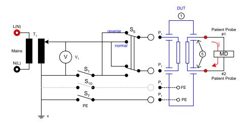
Figure 7.0: Patient Auxiliary Current (Figure 17 of IEC60601-1)
