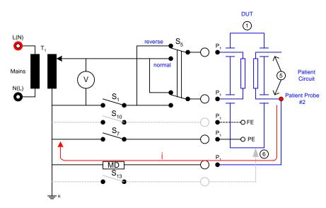
Figure 4.0: Patient Leakage - Applied Part to Ground (Figure 14 of IEC60601-1)
