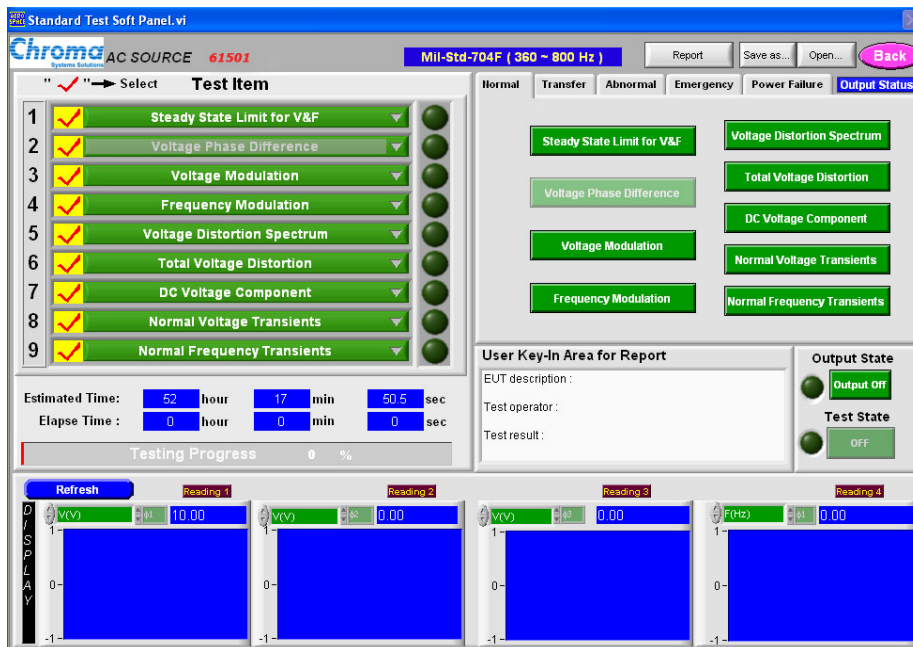
Figure 10. Mil-std-704 Test Screen for Variable Frequency Test
