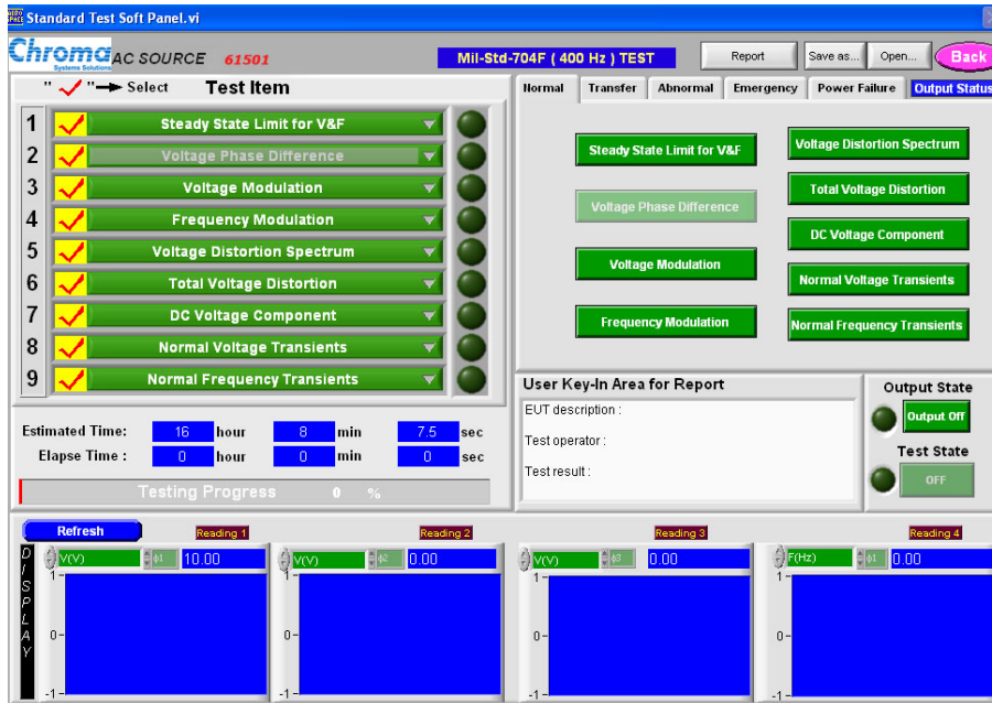
Figure 9. Mil-std-704 Test Screen for 400Hz Test
