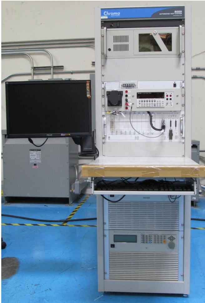
Electric Vehicle Supply Equipment (SAE-J1772) Test System
