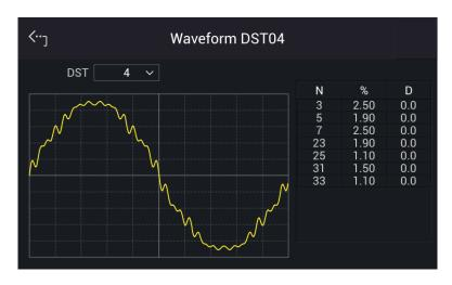
In Meas. & Setup (3\_Phase Mode/1\_Phase Mode) main page, set the Vac to 100.0V, and then tap **ON/OFF** to enable the waveform.
