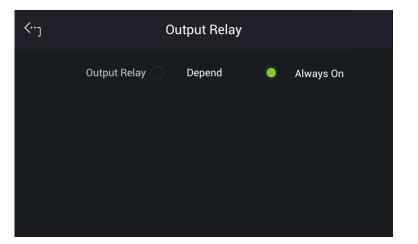
Select "Always ON" for Output Relay to complete the setting.
