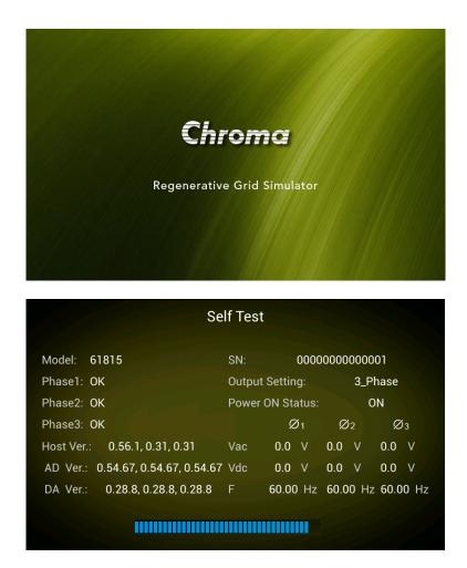
During initialization, the Regenerative Gird Simulator executes memory, data, and communication self-tests. The display shows the Model Number and Regenerative Gird Simulator's Serial Number after executing the self-test routines and each test item will show "OK" on the right if no error is found. The software version will show on the display.
