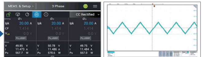
In PU mode, the peak current can be set by the user.
