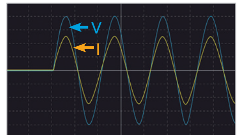
Fast Standby Startup Loading Test
