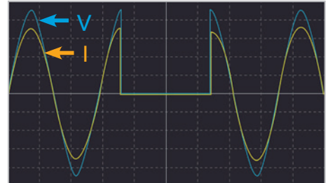
Voltage Interruption Load Test in CR Mode
