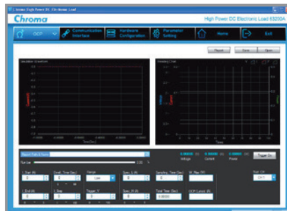
Over Current Protection
