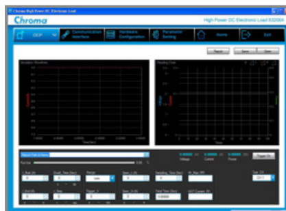
Over Current Protection
