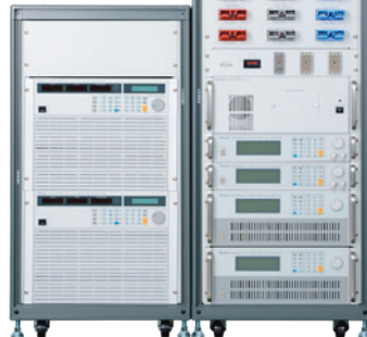
Integrated BMS Test System (16S)
